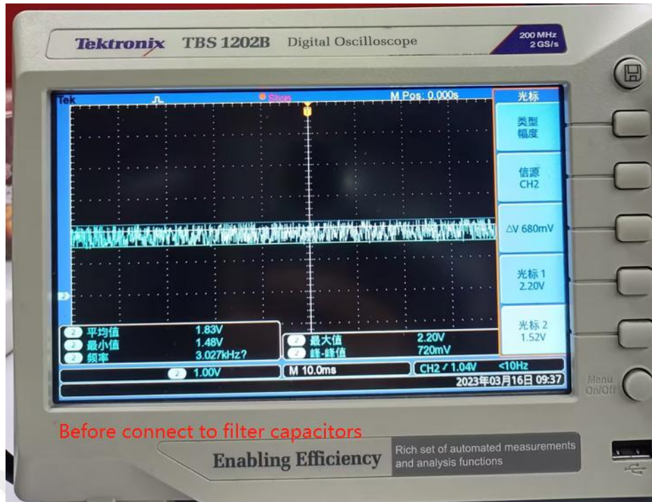
Figure 26: The ripple of RGMII IO power supply before connect the filter capacitor
